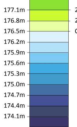
2050 WATER LEVEL WITH FREEBOARD 2050 PROJECTED HIGH WATER LEVEL CURRENT HIGH WATER LEVEL
